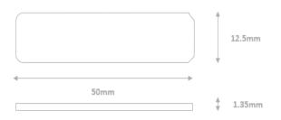
Dimensions stated in mm Supply format = 900 labels per roll
