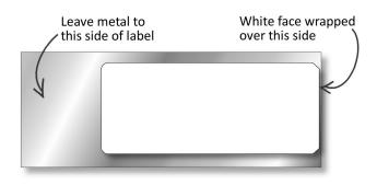
Smallest recommended bending diameter of the Confidex Silverline Blade II<sup>™</sup> is 100mm. For optimal performance please bend the label in the orientation shown below.
